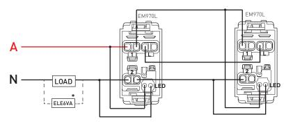
LED Indicator ON when Load OFF Active and Load at first Switch
